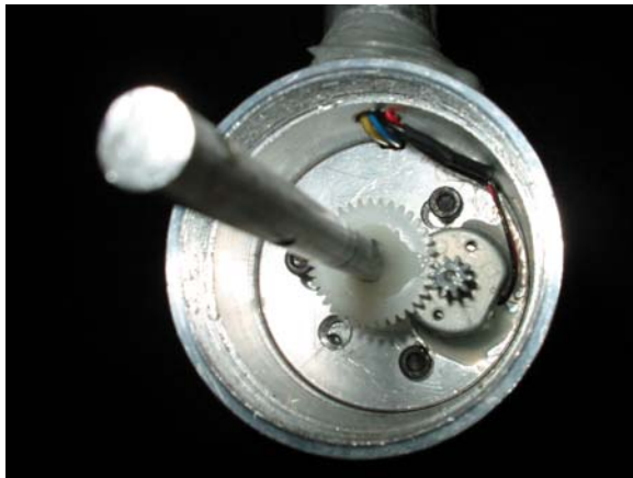
Figure 9 Feedback motor in thruster body
