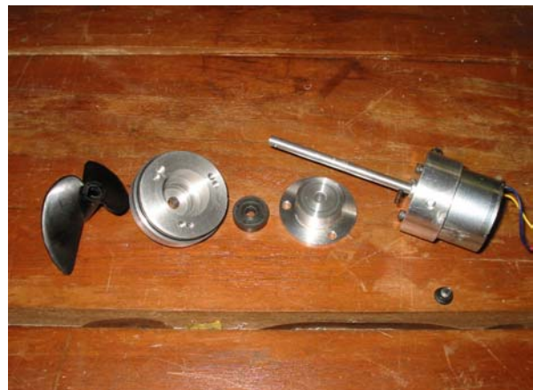
Figure 6 Some parts of the thruster
