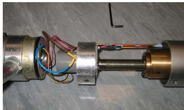
Figure 12 The piston detail
